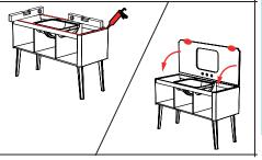
We recommend the use of a silicone adhesive of the same colour as the countertop. Make sure to apply a generous amount of silicone to all surfaces as shown in the diagram and remove any excess once the countertop has been fitted. Allow to cure for as long as indicated in the manufacturer's instructions.
